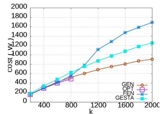
Figure 1: Performance vs. number of pairs on a synthesized internet topology, with  $T = 6$ . Edge weights are uniformly distributed on  $[1, 10]$  to simulate an additive Quality-of-Service metric.
