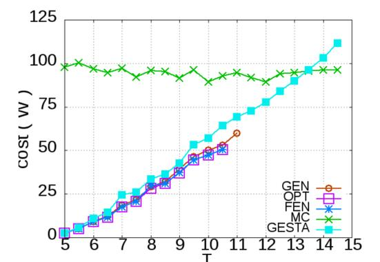
Figure 2: Performance vs. threshold  $T$ , for  $k = 1$ . MC is minimum-cut algorithm. All results are averaged over 10 choices of  $\mathcal{S}$ . This experiment is on an Erdos-Renyi random graph with  $|V| = 1000$ ,  $|E| = 49995$ .
